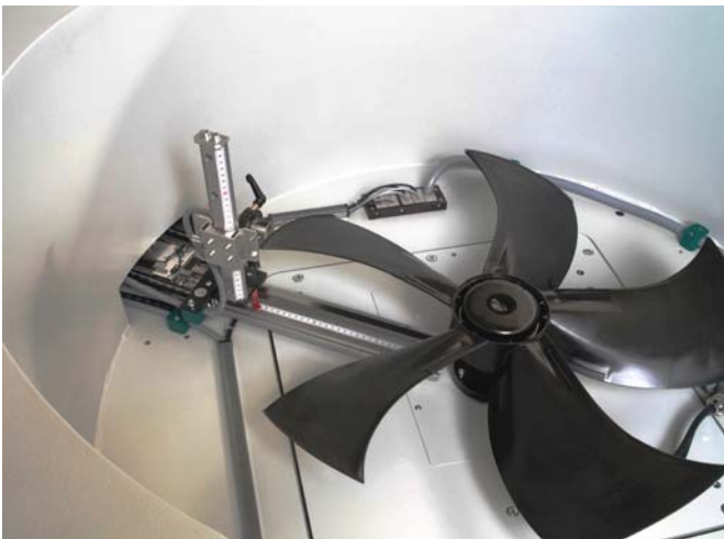
Placement of a 700 mm axial blower
