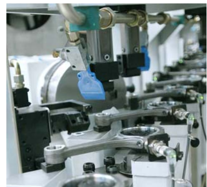
Milling and deburring of small-end All information without obligation, subject to change without notice
