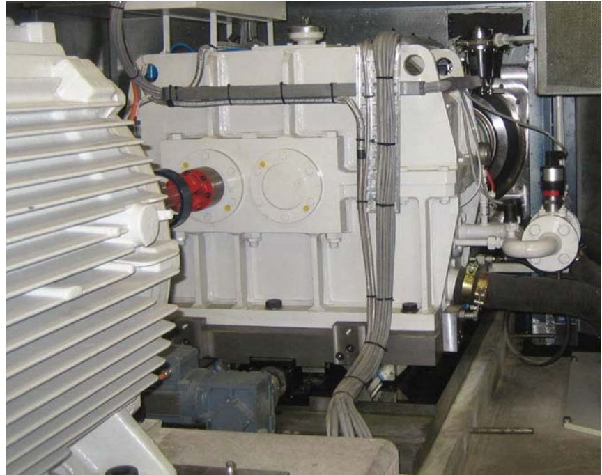
Drive system with motor, gear box, intermediate shaft and moving device
