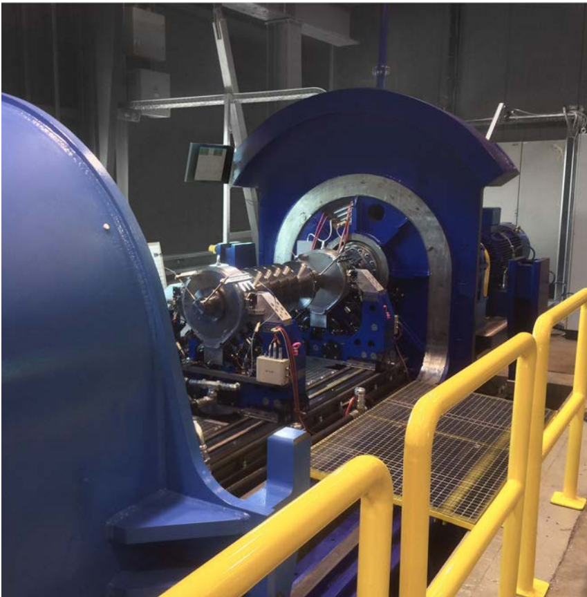
High-speed balancing installation HS 23 with vacuum proof safety containment to balance centrifugal compressors
