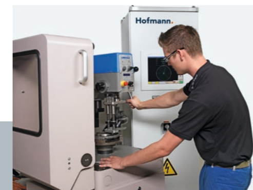
Balancing of a customer rotor at Hofmann
