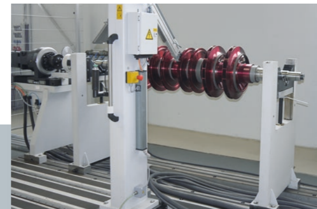
Runout inspection of turbo compressor
