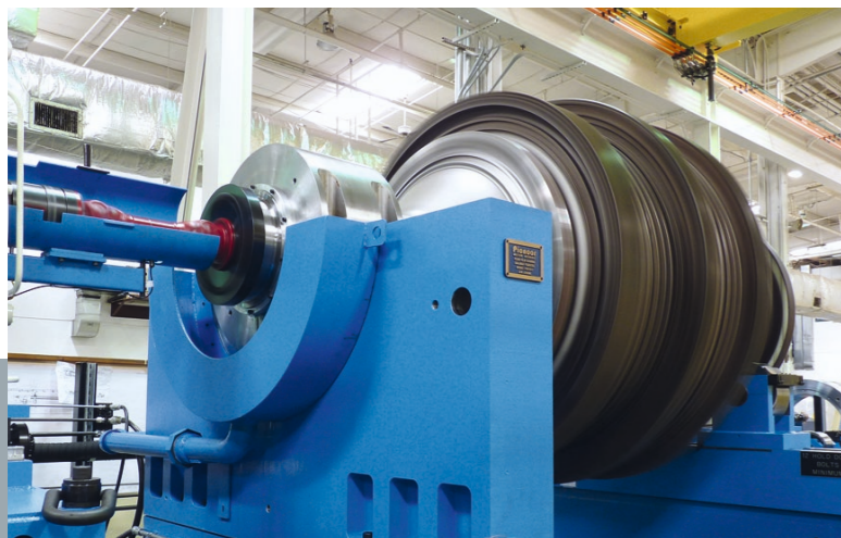
Balancing machine with journal bearings for gas turbine rotors up to 100 tons
