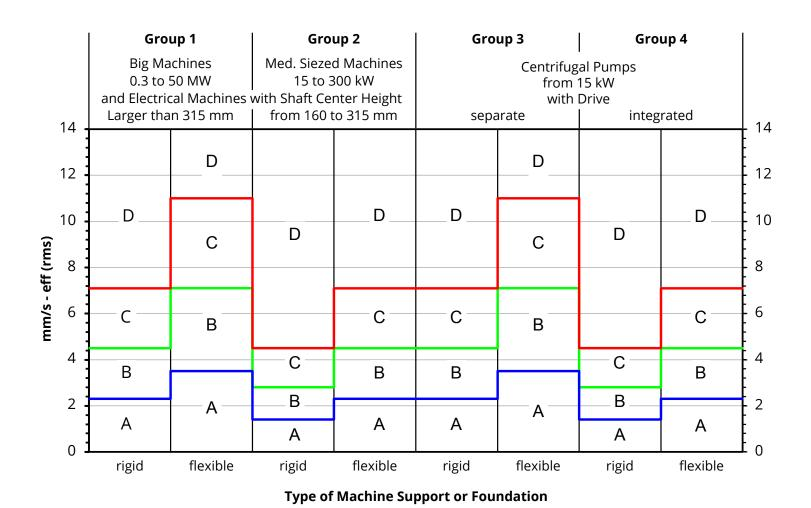
Zones: A = New Machine, B = Applicable for Continuous Operation C = Stop in Near Future, D = Dangerous
