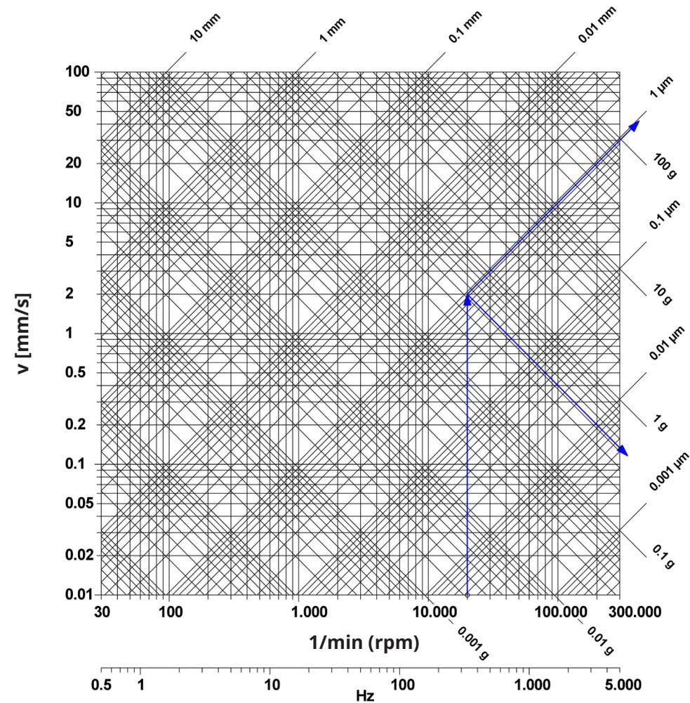
Example: 2 mm/s vibration velocity at 20,000 rpm comply with appr. 0.95  $\mu\text{m}$  vibration displacement or 0.42 g vibration acceleration
